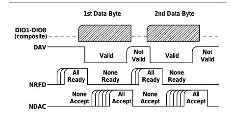
Figure 1-2. Typical GPIB Handshake Operation
