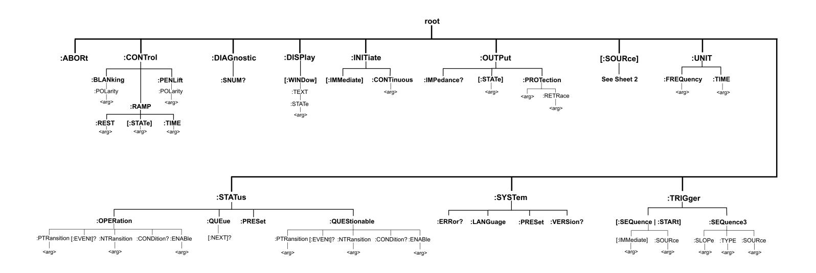
Figure A-1. Overall MG369XA SCPI Command Tree (Sheet 1 of 2)
