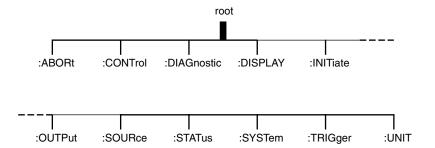
All MG369XA SCPI commands, except the ABORt command, have one or more subcommands (keywords) associated with them to further define the instrument function to be controlled. The subcommand keywords may in turn also have one or more associated subcommands (keywords). Each subcommand level adds another layer to the command tree. The command keyword and its associated subcommand keywords form a portion of the command tree called a command *subsystem*. The :CONTrol command subsystem is shown below.
