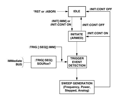
Figure 2-2. MG369XA Trigger Model
